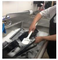
3. Utilizing a scraper, scrape all dry residues and any buildup. Remove buildup using a vacuum.
