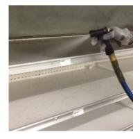
8. Select 'Sanitize' on MiniChem unit and attach foam wand. Spray interior of case with Q-San 7.5. Allow 1 minute of contact time.
