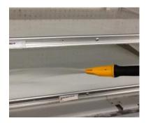
9. Select 'Rinse' on MiniChem unit and attach Foam San. Spray the lower housing of the sales case with Foam San (no need to rinse off).
